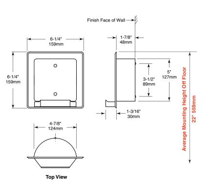
Rough Wall Opening: 5-1/4" (133mm) Wide 5-1/4" (133mm) High 2" (51mm) minimum recessed depth
