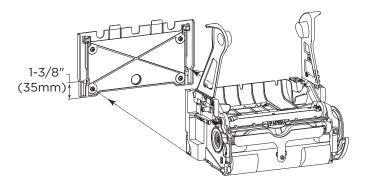
Place the 3974-356 module on that location, ensuring that both sides of the module are flat against the Module Mounting Plate and engages with the slots on both sides and push the module down until the tabs lock it into place.
