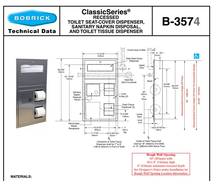
Cabinet — 18-8, Type-304, heavy-gauge stainless steel. All-welded construction. Exposed surfaces have satin finish.
