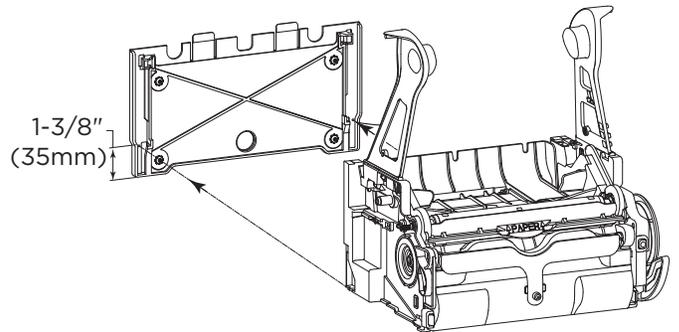
Place the 3974-356 module on that location, ensuring that both sides of the module are flat against the Module Mounting Plate and engages with the slots on both sides and push the module down until the tabs lock it into place.
