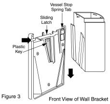
3. While pushing in again on the concealed sliding latch and pushing back on the vessel stop, spring tab, slide the wall bracket down to separate it from the soap vessel.
