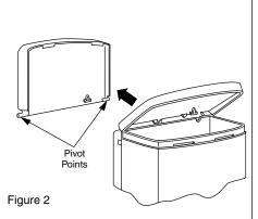
2. Remove the lid by swinging it up to the full vertical (open) position, then sliding it directly back off the wall bracket.
