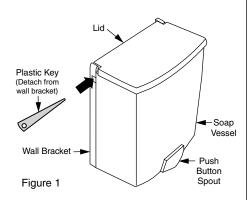
1. Break off the plastic key from the wall bracket (see Figure 3). Using this key, push the concealed sliding latch located in the small slot at the upper left side of the wall bracket. The lid will automatically pop forward.
